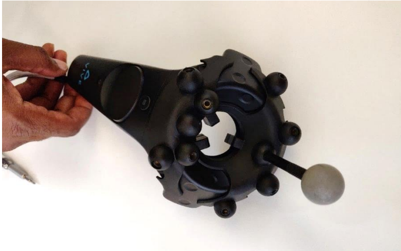
Figure 28 - Tracking markers are attached to the holder using a standard M3 distance rod.
