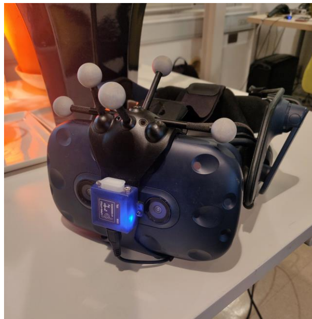
Figure 25 - Fully assembled VIVE Pro LPVR holder
