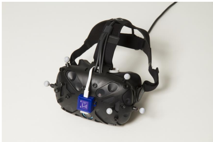
Figure 24 - The fully assembled VIVE LPVR holder.
