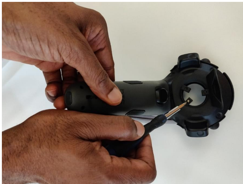
Figure 27 - Align the holder components with the hand controller as shown in the image and connect them using the screws delivered with the set.
