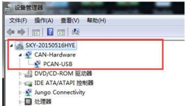
When the hardware setting of PCAN-USB is completed, users can connect it with LPMS-CANAL2 sensor with proper wiring between the M12 and DB9 connectors. Then the PCAN-USB can be plugged into PC to power the sensor and acquire data.
