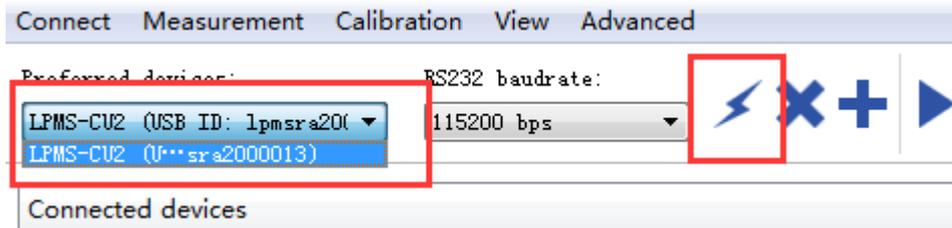
After completing all the steps above, the LPMS-CU2 should have been connecting with windows system. Users can check all the data visualization and parameter settings of the sensor from LpmsControl.
