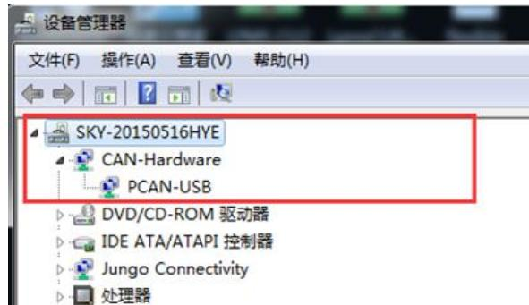
When the hardware setting of PCAN-USB is completed, users can connect it with LPMS-CU2 sensor. Then by plugging the PCAN-USB to PC, the LED on the sensor should behave like a pulsating light at blue color, which indicates the sensor is functionally working.
