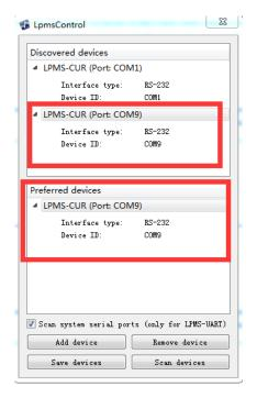
6) To select the target sensor ID from the Preferred devices list, and click Connect function under "Connect" menu or click the lightning button on toolbar to connect the sensor. Note: The default baudrate of RS232 communication is 115200bps.
