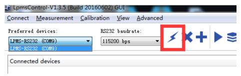
After completing all the steps above, the LPMS-RS232AL2 should have been connecting with windows system. Users can check all the data visualization and parameter settings of the sensor from LpmsControl.
