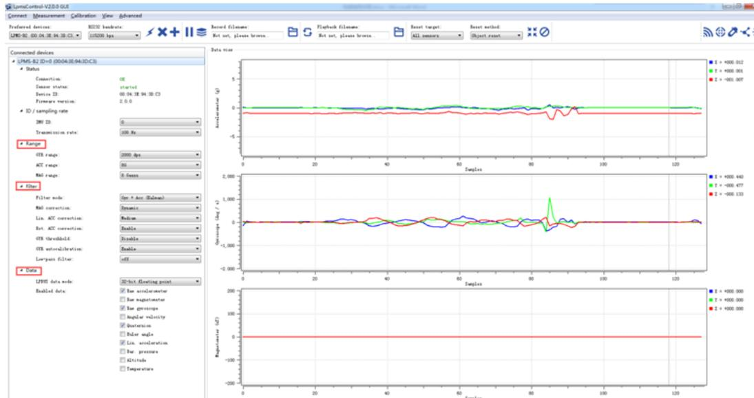
On the left side of the main interface of LpmsControl, users can change the sensor settings, like measurement range, filter modes, data updating rate, etc. Moreover, the types of output data can be modified by checking or unchecking the check box of each parameter. For example, in the following image the "raw magnetometer" is checked so that the acquisition of magnetic data is enabled.
